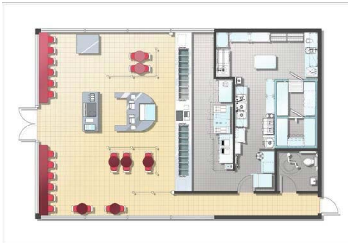
Figure 4. Example of a fast-food restaurant layout with all required sections and functions
